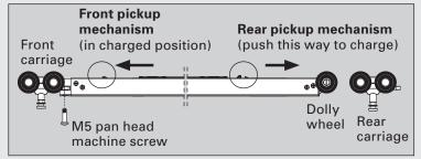
a) The twin SofStop mechanism fits together as shown above. Push front and rear pickup mechanisms in the direction shown to charge.
