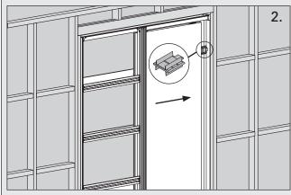
Hold setting block on closing jamb/finished wall and gently close door. Activator will slide to correct position. Securely tighten set screws on activator.
