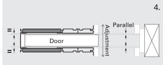
Check that door slides parallel and straight. Adjust if necessary.
