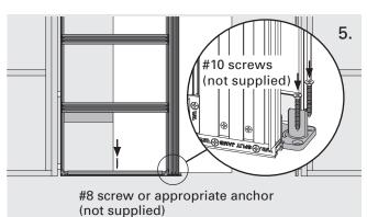
Securely fix T-Guide then bottom plate to floor
