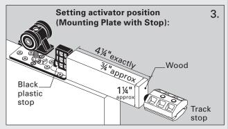
Cut piece of wood to 4-1/4" (108mm) and insert it above door, hard up against black plastic stop on mounting plate. Slowly close door until wood hits rubber part of track stop. Open door and securely tighten set screws on activator.
