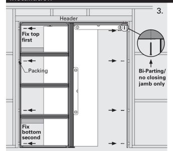
Keep plumb and pack where required. Fix back stud and closing jamb (if using) with #8 countersunk screws (not supplied).
