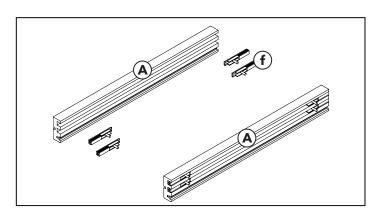
Step 3 Cut the jamb headers ( $\bf A$ ) into two lengths equal to the space remaining between the split jambs ( $\bf B$ ). Insert the bolts ( $\bf f$ ) (4 pcs on each header piece).
