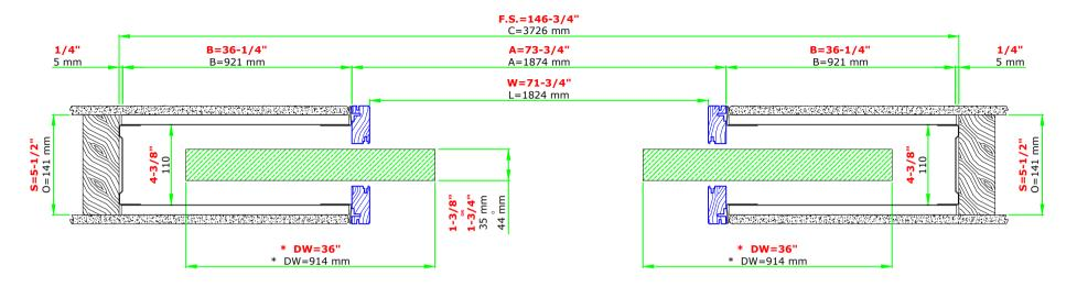
\* Door panel width could be increased by 1" to keep the door on the floor guide at closed position, alternatively using the Anti Warp Profile (sold separately) on std size doors but made longer to stay on the guide.
