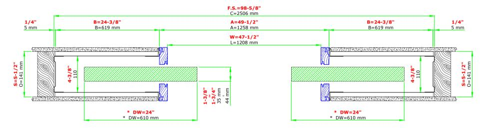
\* Door panel width could be increased by 1" to keep the door on the floor guide at closed position, alternatively using the Anti Warp Profile (sold separately) on std size doors but made longer to stay on the guide.
