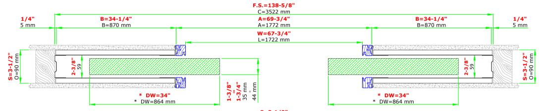
\* Door panel width could be increased by 1" to keep the door on the floor guide at closed position, alternatively using the Anti Warp Profile (sold separately) on std size doors but made longer to stay on the guide.
