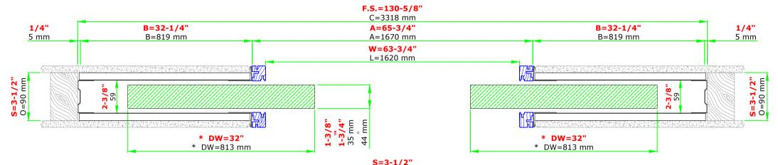
\* Door panel width could be increased by 1" to keep the door on the floor guide at closed position, alternatively using the Anti Warp Profile (sold separately) on std size doors but made longer to stay on the guide.
